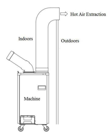
\* Extended hot exhaust pipe shall be separately purchased from the Company specification shall be  $\Phi$ 160x3m.
