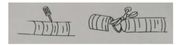
• Method of Reducing the Diameter of Extended Pipe
